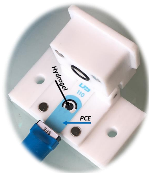
Figure 4.1 Electrochemical reduction of P(\text{TEMPO}^+-r\text{-OEGMA}) hydrogels, swollen in aqueous \text{NaClO}_4 and loaded with aspirin using the printed carbon electrode method (PCE).
