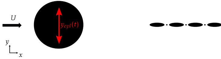
Figure 5.9: Simulation setup: cylinder of diameter D moving in the y direction.
