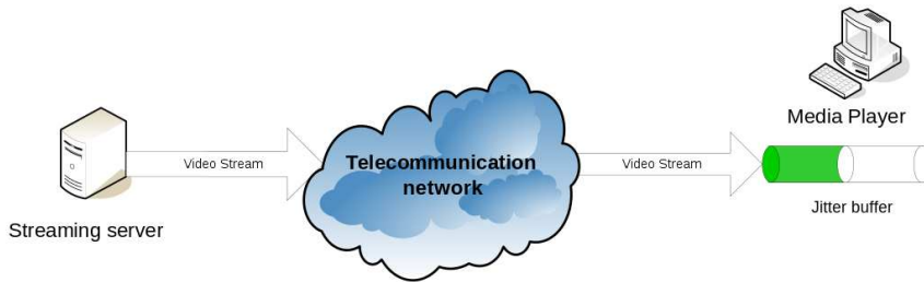
Figure 1.1: Typical streaming chain
