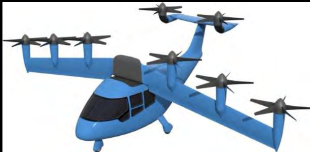
Tilt-Wing (Airplane mode for efficient cruise flight, helicopter mode for VTOL) [4]
