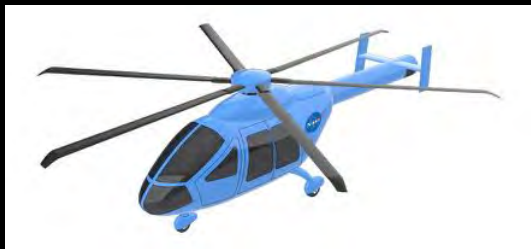
Quiet Single-Main Rotor (QSMR) (NOTAR, specifically designed for quiet operations) [3]
