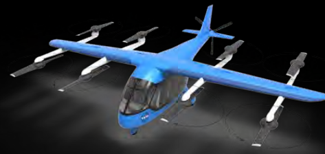
Lift+Cruise (Hybrid-Mounted Rotors)
