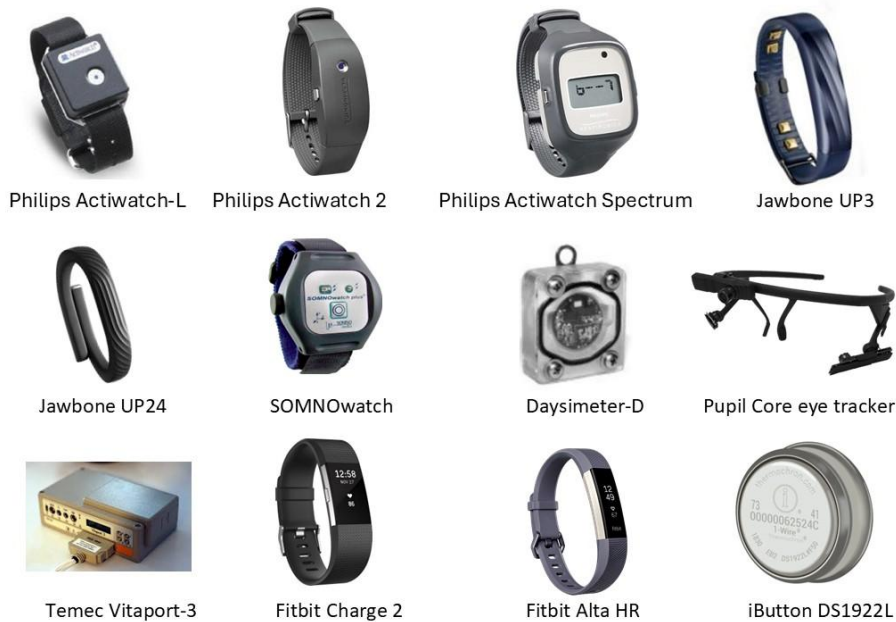
Figure 6. Exemplary selection of the hardware used for physiological and human activities monitoring.
