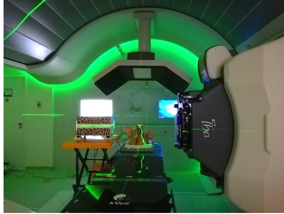
Figure 2: Experimental setup. The MLIC was placed on a lift table and aligned with the laser system.
