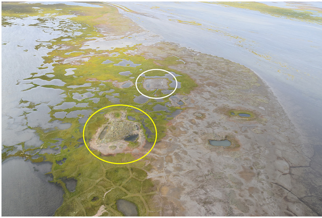
FIGURE 9 | Waste disposal sumps at the Mallik site, outer Mackenzie Delta, Northwest Territories. The sump in the foreground in the yellow circle is Mallik L-38, constructed in 1972. The sump in the middle distance circled in white was built in the 2000s for use by several projects [82]. Photograph by Tim Ensom, 2022. [Colour figure can be viewed at wileyonlinelibrary.com ]
