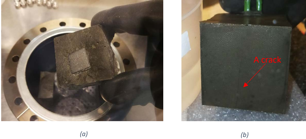
Figure 6. Pictures showing (a) the breach of a GC sample in condition 1 after 133 days and (b) a crack in an EC sample appeared in condition 2 generated after 8 days.
