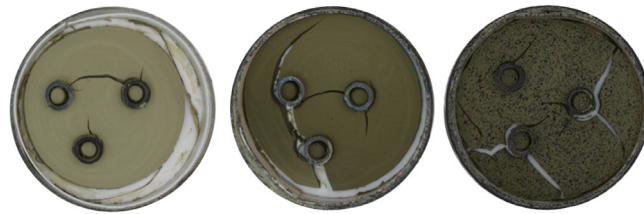
Fig. 25. Different crack patterns observed for the same configuration with 3 inclusions.
