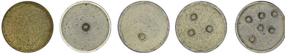
Fig. 1. Experimental samples: S_0 , S_{1c} , S_1 , S_3 and S_6 . Underscript c indicates that the inclusion is centered.
