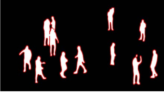
Figure 2. The Beucher gradients of the masks produced by \mathcal{T} define thin margins (in red) whose pixels are excluded from the quantitative evaluation process in order to reduce the impact of the lack of accuracy of \mathcal{T} at the borders of the masks on the evaluation.
