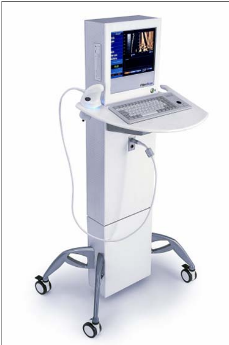
Figure 4. The FibroScan is a dedicated machine that is composed of a probe and a control unit. The probe includes an ultrasonic transducer mounted on the axis of a vibrator (From: EchoSens, Paris, France).
