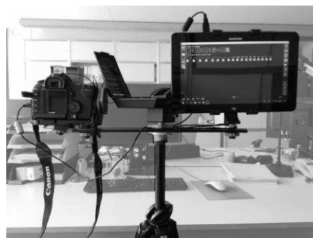
Figure 2 – Study equipment set-up: camera and fisheye lens, vertical illuminance sensor, and tablet computer on a tripod
