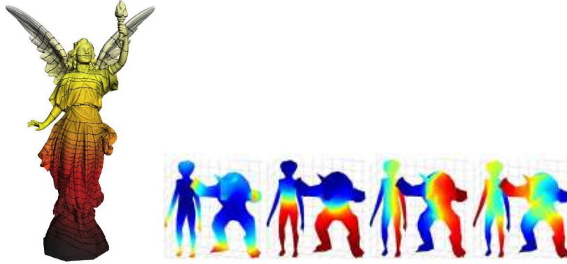
Figure 7.4: Vibration modes on 3D meshed models. On the left, the Fiedler vector isovalues have been color coded. Isenburg et al. propose to use it to stream meshes from an extremity to another (image courtesy of Isenburg et al. [64]). On the right, the first non constant vibration modes have been represented with colors. These are the four first non-constant eigenvectors of the KL operator for two different models. It can be seen that these similar shapes also have similar eigenvectors.
