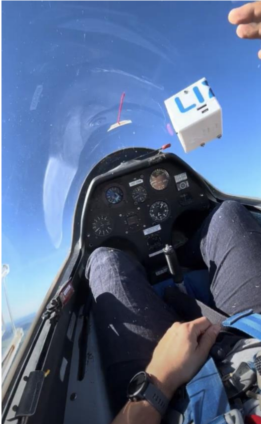
Figure 1: Experimental object in microgravity during a parabolic flight in a glider.
