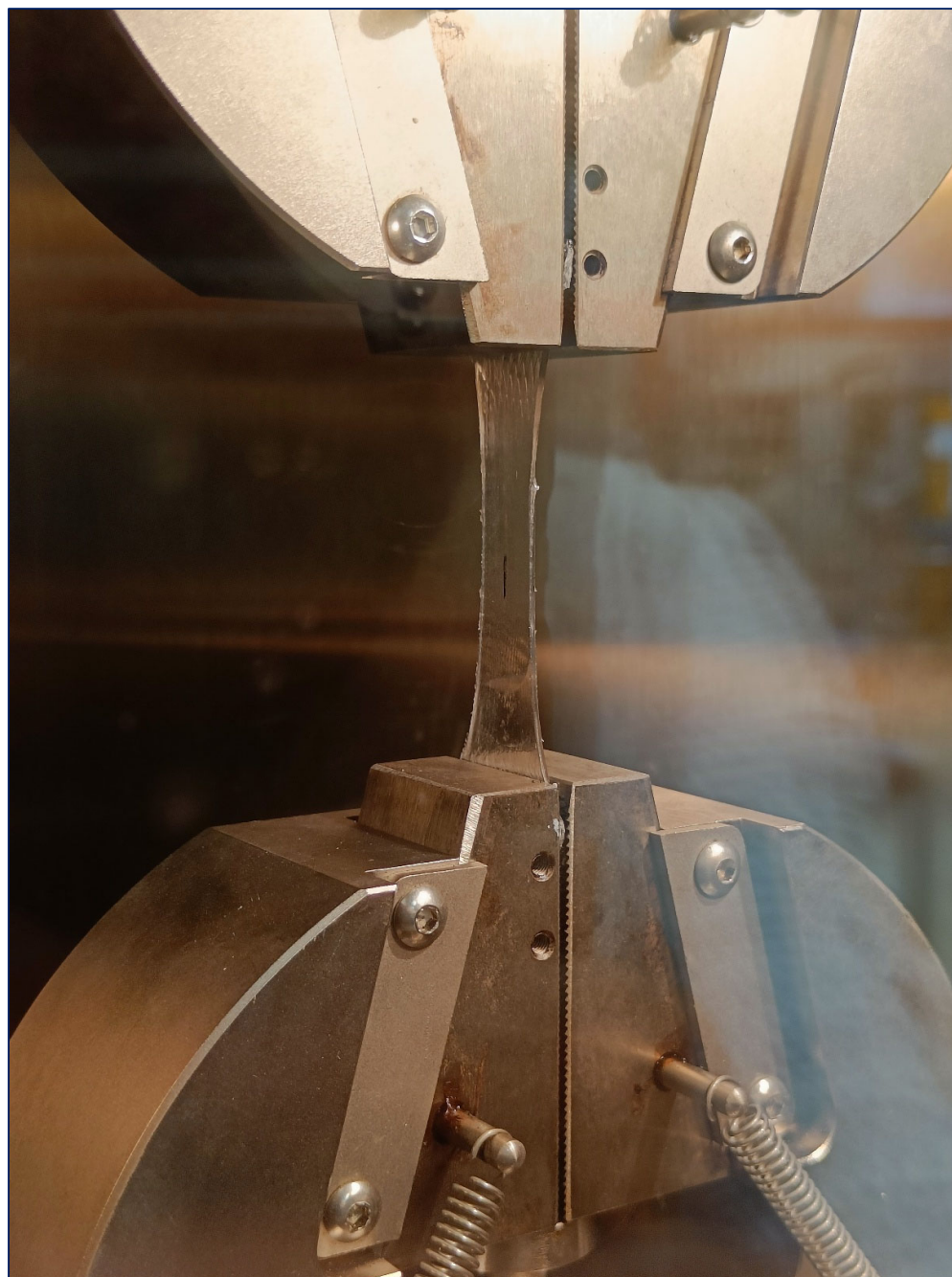
Figure 1. Experimental setup for tensile extensional rheometry. The image, captured through the oven window (note reflections), shows the sample at 130°C during a test at a Hencky strain rate of 0.03 \text{ s}^{-1} , at a crosshead displacement of 40 mm ( \varepsilon_h \approx 1.4 ). The fixture, clamps, and the deformation of a central (black) marker are visible.
