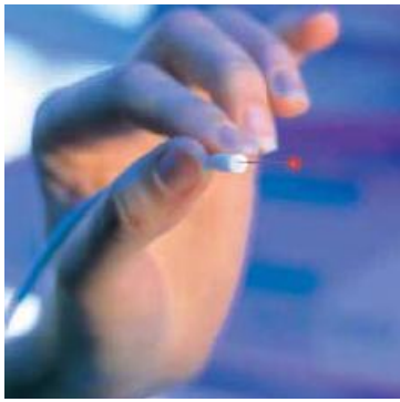
Figure 7: Optical probe induces pulsatile fluorescence (A) and Oxylite device capable of continuous, quantitative measurement of dissolved partial pressure of oxygen (B).
