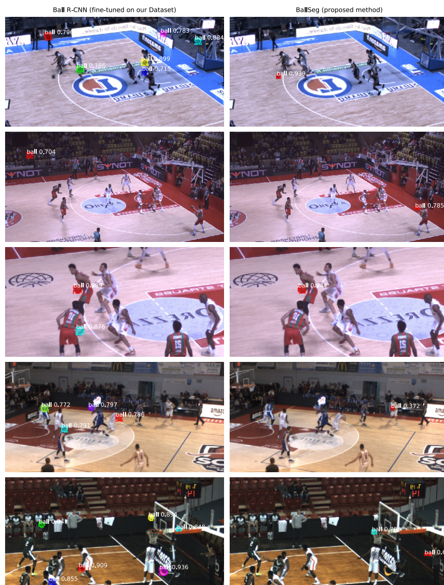
Figure 4.5: Comparison of our BallSeg with Ball R-CNN . BallSeg gives accurate results in many different configurations, with fewer false positives.
