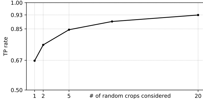
Figure 4.6: Detection rate using test-time data-augmentation. 1000 random-crops were created for each scene. Ball detection rate as a function of the number of random crops considered for a scene, for a top-1 detection rule. The ball is detected in the scene if it is detected in at least one of the random crops considered.
