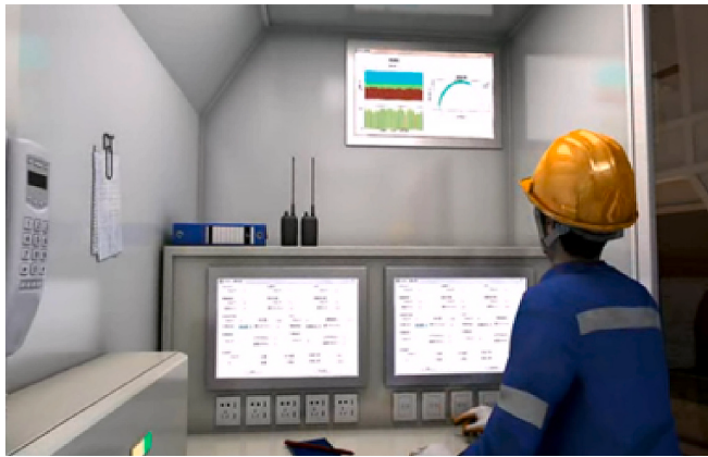
Fig. 22. The automatic operation of GPR Monitoring System on tunnel construction site.
