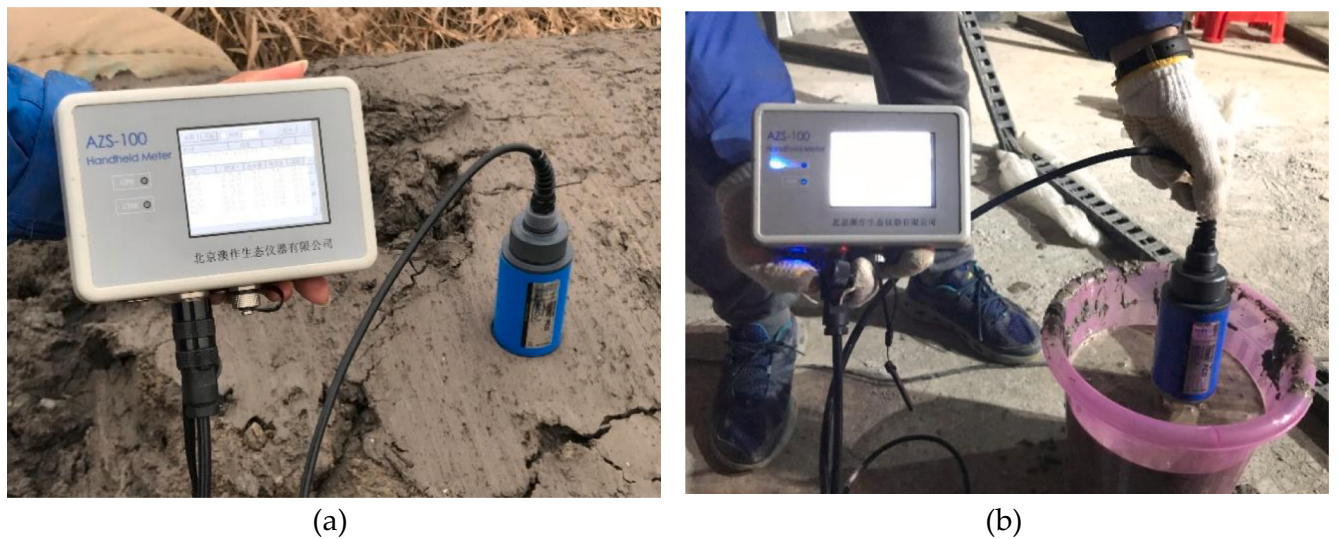
Fig. 12. The dielectric constant and conductivity tests on (a) re-backfilled soils and (b) grouting materials.
