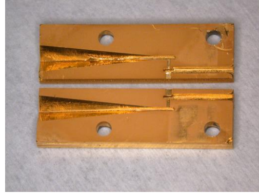
Fig.5. Image showing embossed gold coated polymer w/g block
