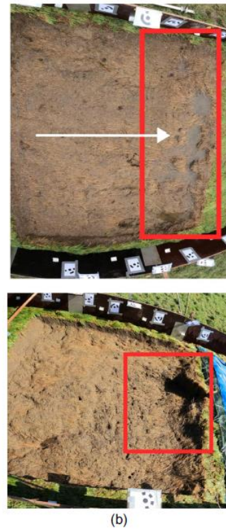
Fig. 13. (a) Photogrammetric verification versus RTK measurements for multicamera set-up at section BC2-2; (b) water-shadow negative effects.
