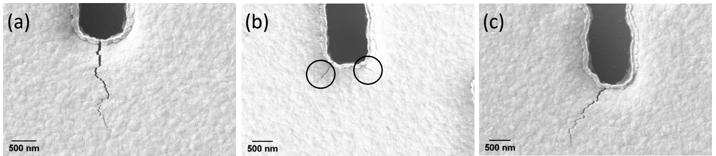
Fig. 5. Selected SEM micrographs of COC test structures illustrating different crack propagation behaviors leading to scatter in fracture toughness values: (a) crack deviation due to the “microstructure effect”, (b) initiation and propagation of two cracks due to the “stress state at the notch front effect”, (c) side crack propagation due to the “misalignment and notch effect”.
