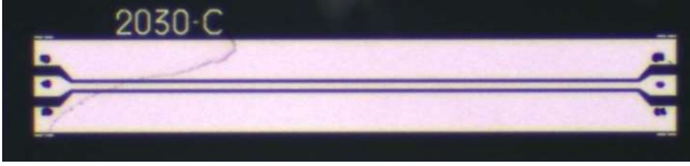
Fig. 4. CPW lines for proposed PSi characterization (signal width, ground spacing and ground width of 26, 40 and 155 \mu\text{m} respectively).
