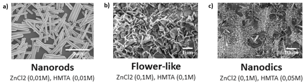
Figure 3.1.: SEM images of ZnO nanostructures (prepared by liquid phase synthesis using zinc chloride and hexamethylene tetramine as precursor in the water) deposited by varying the concentration of the reactant (a) nanorods, (b) flower-like, and (c) nanodiscs- like structures.
