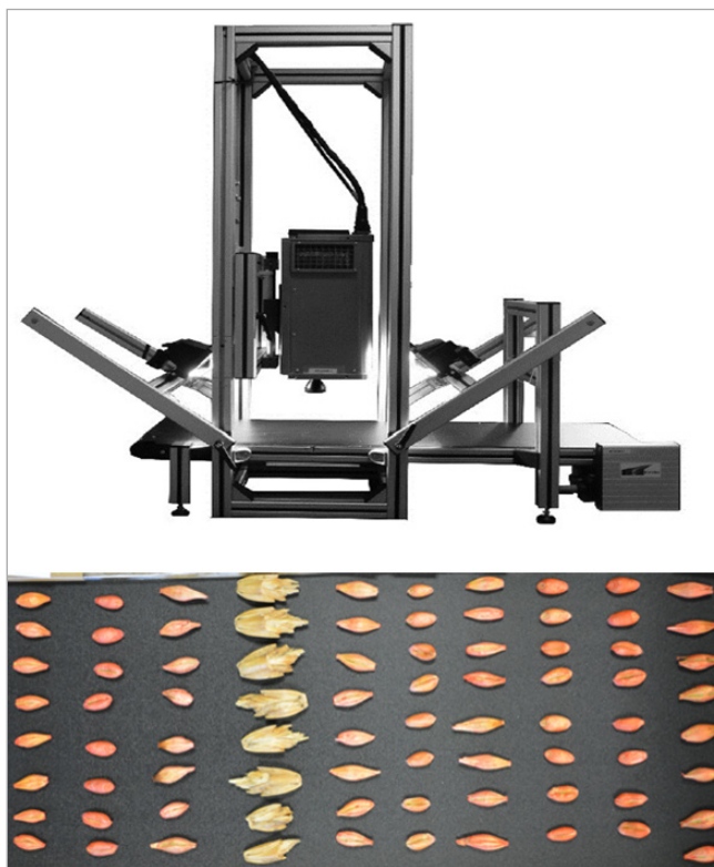
Figure 1. NIR hyperspectral imaging system and multi seeds presentation to the conveyor belt (eight seeds per sample).
