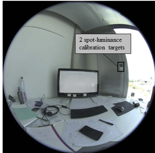
Fig 15 Example of a visual scene with two mid-range grey cards used as targets for spot luminance measurement.
