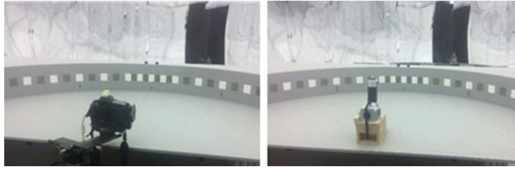
Fig 9 Setup of the equipment for the first method to evaluate the vignetting curves.
