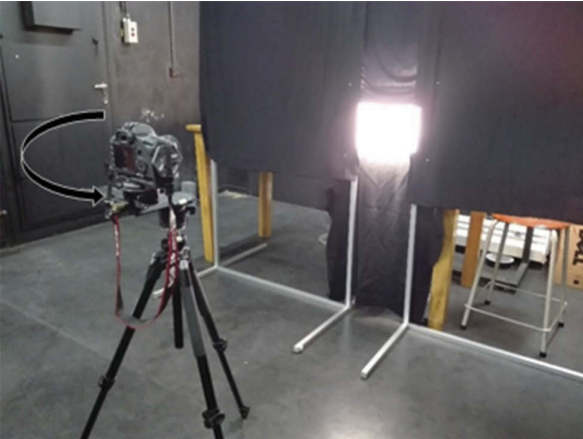
Fig 10 Setup of the equipment for the second method to evaluate the vignetting curves.
