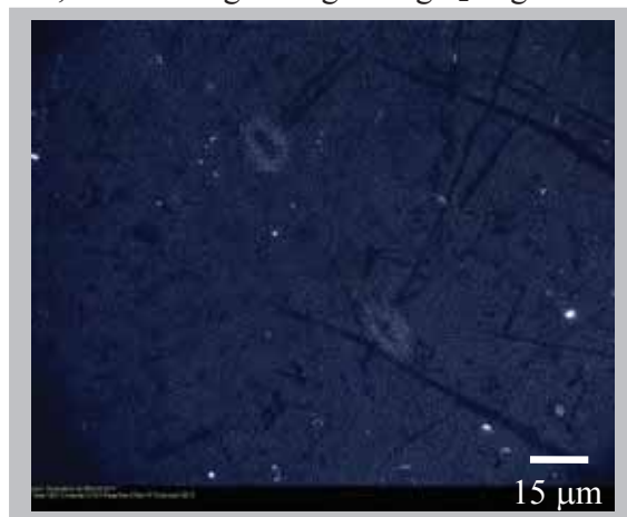
Figure 1. Optical microscopy image showing incipient growth of abundant \text{MgH}_2 nuclei in Mg-Ti layers at 120°C under a \text{H}_2 -pressure of 10 mb.
