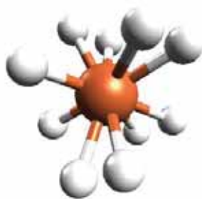
Figure 1, Theoretically predicted structural model of Fe 1 H 10 [1].
