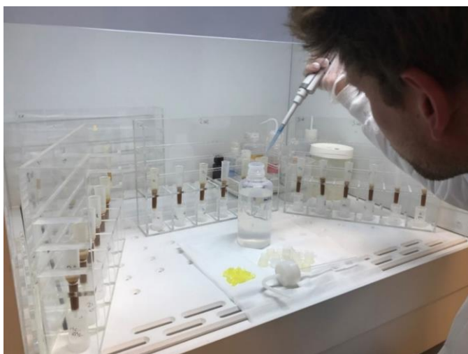
Fig. 2.4: Samples purification via cation-exchange resin (Biorad AG50WX12) prior to Si isotope measurements.
