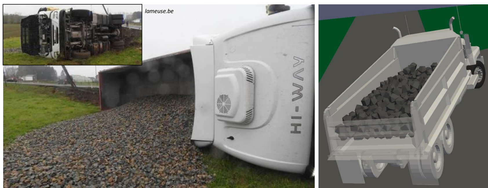
Fig.3 Truck lying on its side following a loss of control maybe caused by the payload.
