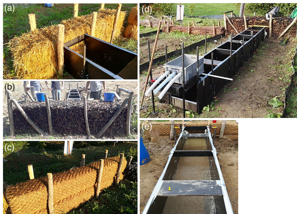
FIGURE 1 Types of vegetative barriers studied: (a) straw bales; (b) wood-chips; (c) coconut-fibre bales and (d) experimental setup to simulate sediment-laden runoff events, also showing the flume fitted to the barrier and the earth dam ponds at each side of the flume. (e) Sediment deposited in the flume after an experiment, also showing ponded water [Colour figure can be viewed at wileyonlinelibrary.com ]
