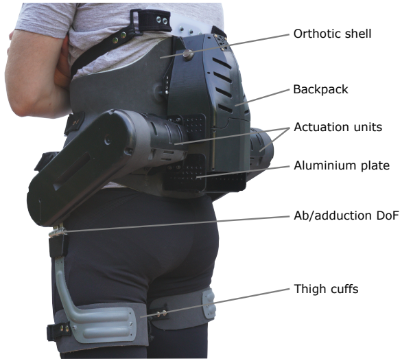
Figure 3.1 The Active Pelvis Orthosis developed in the framework of the CYBERLEGs and CYBERLEGsPlusPlus research projects, now brought to a commercial product by the company IUVO (Pisa, Italy, www.iuvo.company ).
