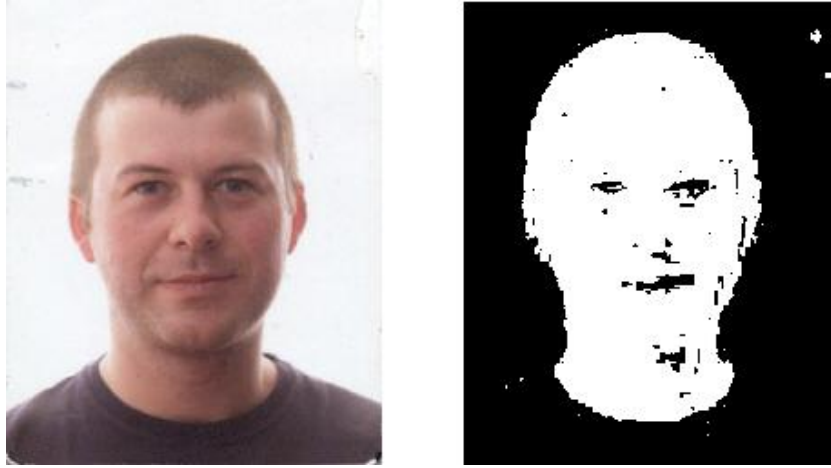
Figure 4.3: The result of a hue-based face detector
