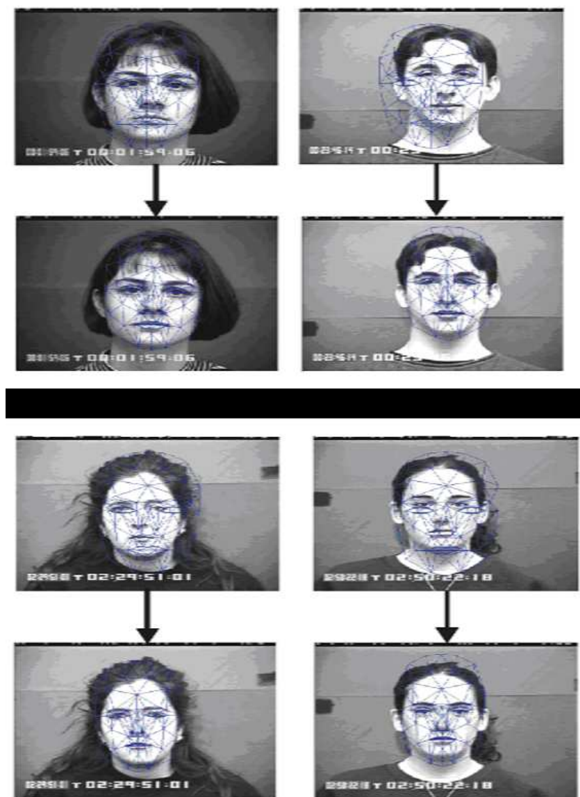
Figure 4.18: The initialization procedure with 10 feature points (4 points for the mouth, and 3 for each eyebrow)
