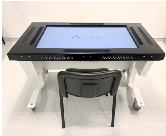
Fig. 1. The non-immersiveVR device. REAtouch® (Axinosis®) touch-sensitive 43" screen tablet with multisensory and real-time performance feedback. The height and inclination of the screen can be adjusted. In the present study, the inclination was the same as that presented here (i.e., 0°).
