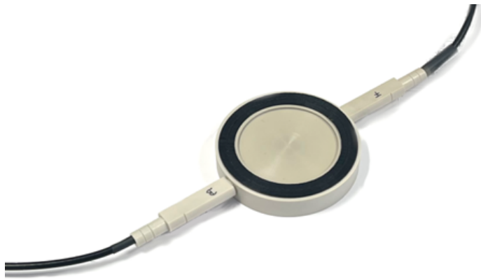
Figure 5.1: External appearance of a DGIC prototype. The dimensions are comparable to those of a standard ionization chamber, though the chamber outer diameter is slightly larger (64 mm) to facilitate prototype assembly.
