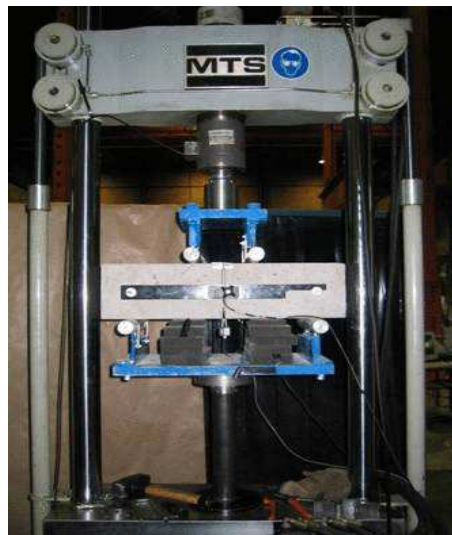
Figure 5.3: Test setup of four-point bending.
