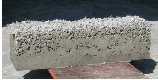
Figure 5.7: Porosity increase of sample with high content of fibers.
