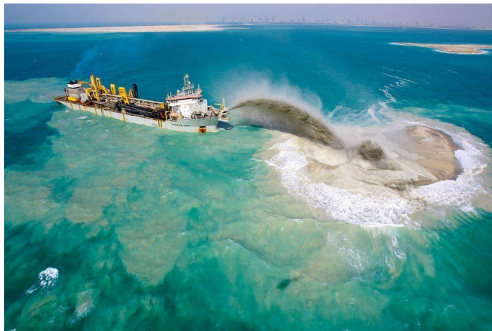
Figure 1.1: The Vasco Da Gama suction-dredging ship in operation. Dredging consists in the aquatic excavation of a granular bed; the increased fluid content of the mobilized sediment allows to easily manipulate it as a fluid.
