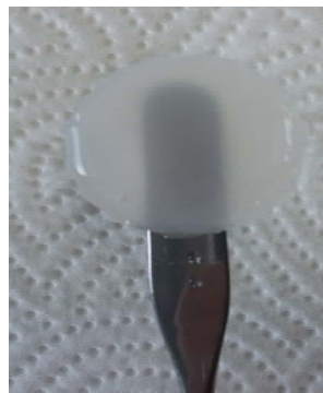
Fig 1. Gelation of alginate hydrogel via diffusion using a saturated with \text{Ca}^{2+} filter paper (a) and the final gelled homogenous alginate (b)
