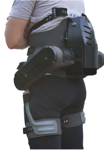
Fig. 1: The Active Pelvis Orthosis developed in the framework of the CYBERLEGsPlusPlus project [8] can deliver oscillator-based walking assistance to the user’s hip. It is now brought to a commercial product by the company IUVO (Pisa, Italy, www.iuvo.company ).
