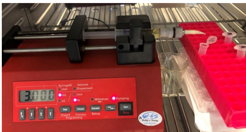
Figure IV-3 Experimental set-up for the transaminations carried out in flow-mode. The whole set-up is working in a drying oven set at 35 °C. The syringe is filled with reaction medium then pushed at a desired flow-rate via a syringe pump. TA immobilized-membrane lies at the junction between the head of the syringe and bottom of the needle. Samples of the outflow are collected in an Eppendorf each 30 minutes.
