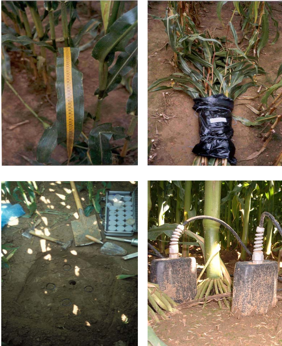
Figure 2.3. 1999 field campaign. Top left: measurement of width and length of about 15 maize leaves on each 280 maize plant. Top right: manual yield of maize for dry matter estimation. Bottom left: in-situ calibration of neutron probe (second phase, i.e. measurement of volumetric soil water content at a given depth with four kopecki rings). Bottom right: TDR probes installed for in-situ calibration.
