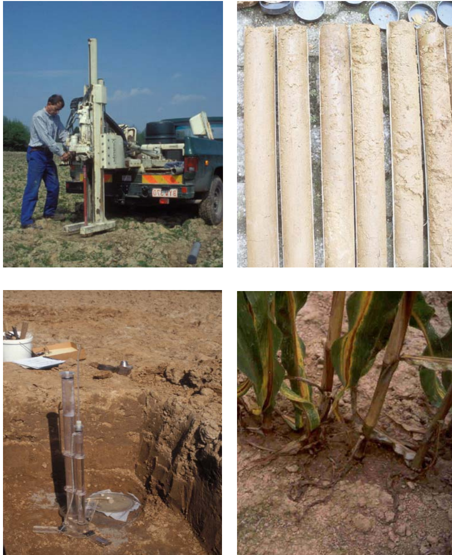
Figure 2.5. Top left: collection of the undisturbed soil columns with the hydraulic auger. Top right: severed undisturbed soil columns. Bottom left: infiltrometer measurement at 50 cm depth (March 2002). Bottom right (2003): visual observation of throughfall under maize canopy after a small rainfall amount of 5 mm (see the difference of soil colour within and between the rows)
