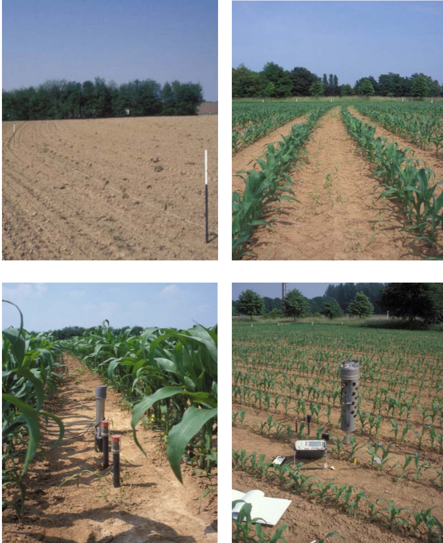
Figure 2.2. 1999 field campaign. Top left: localization of the sampling locations within the experimental field. Top right: growing maize at the end of May. Bottom left: tensiometers, TDR probe and access tube installed mid-way between the 75 cm spaced rows. Bottom right: field measurements with neutron probe, Tektronix, tensimeter and the unavoidable field book.
