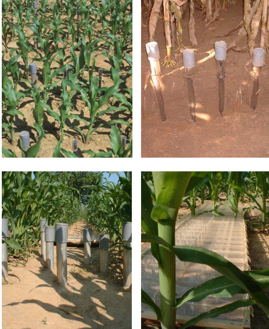
Figure 2.4. Top left (2000 experimental setup): transect of 50 sampling points. Top right: removal of the 2002 PVC tubes. Bottom left (2003 experimental setup): small transect with 14 access tubes installed perpendicularly to three maize rows. Bottom right (2003 experimental setup): measurement of throughfall under the maize canopy.
