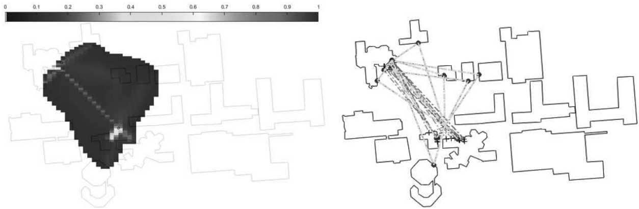
Fig. 8. Left panel: Normalized weights for a given snapshot, for the Saint Barbe route. Right panel: Propagation paths and centroids for the same snapshot. Transceivers are represented with black dots. Dashed red lines are propagation paths. Black crosses represent propagation paths first and last bounces. Blue dots are centroid first and last bounces. Thick green line represent the propagation path of the centroid. There are 24 propagation paths and 9 clusters for the snapshot. Six of the clusters are singleton, one has 2 members, another 7 and another 9.
