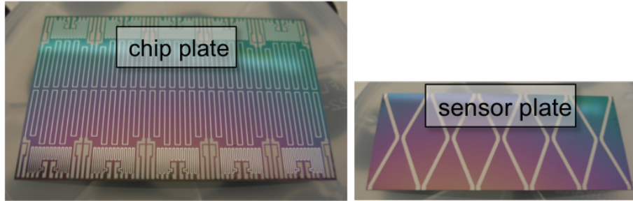
Figure 3.21: Silicon mock-up plates before glue assembly.
