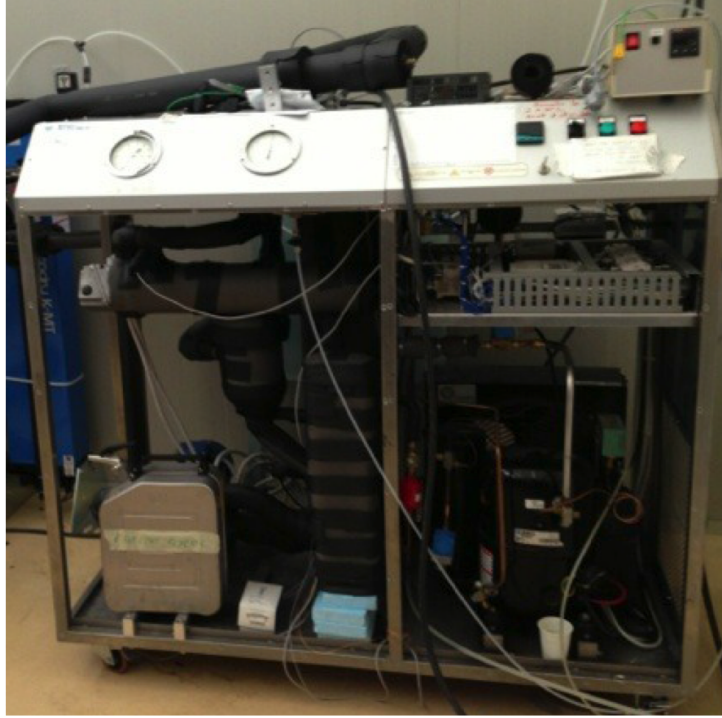
Figure 3.28: CMS pixel test cooling plant.
