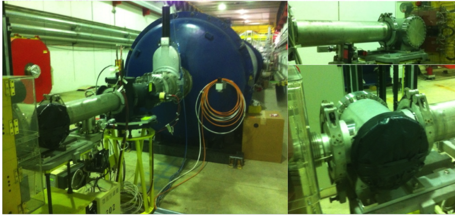
Figure 5.2: GTK housing installed at the position of GTK 3 for the technical run in 2012
