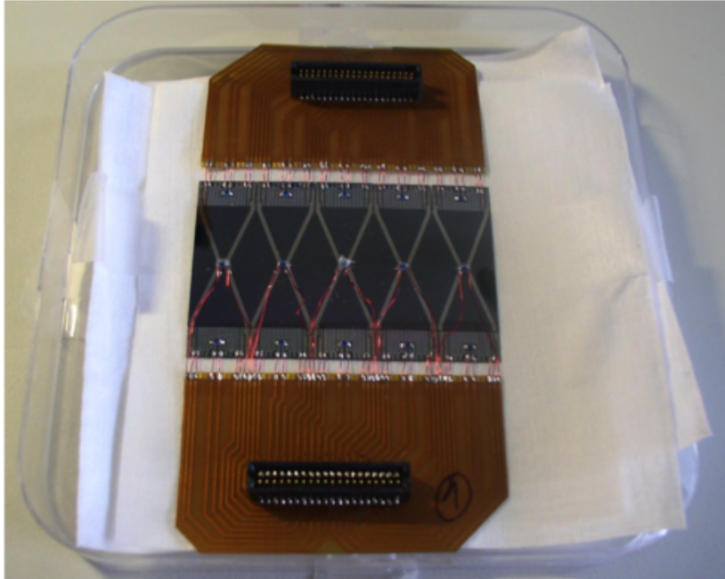
Figure 3.22: Silicon mock-up assembled and equipped with temperature sensors.
