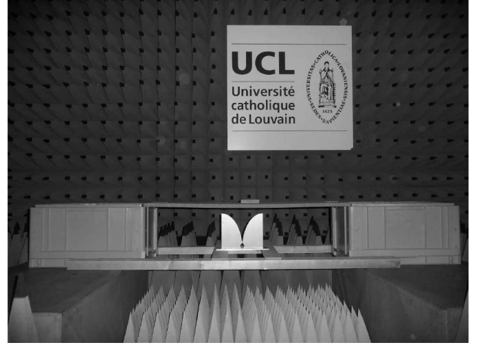
Fig. 1. Experimental setup with a wooden frame supporting the antenna, while plastic boxes support a microwave foam on which the calibration target and OUT may be positioned (the dielectric test object is present in the photo).
