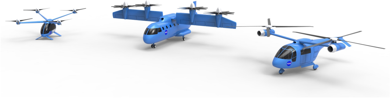
Figure 1: Three UAM vehicle concepts proposed by NASA: quadcopter (left), lift plus cruise (center) and side-by-side (right) configurations. The lift plus cruise vehicle is shown in hover mode. In cruise, the wing and rotors ensemble is tilted down and resemble a conventional airplane. The other configurations operate in cruise as shown. Figure reproduced from Ref. 6.
