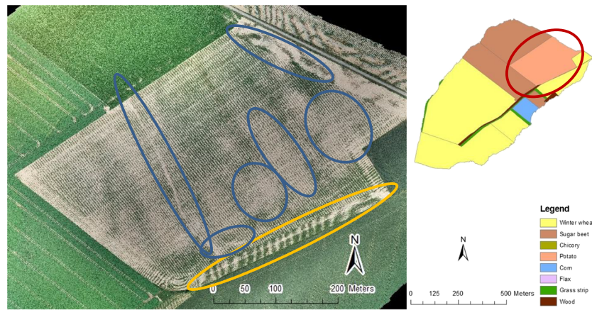
Figure 11. Orthophotoplan of 26 June 2019 after a large runoff event (10 June 2019) and the location of field, ephemeral gullies and deposition sites (blue: erosion sites, orange: deposition sites). [Colour figure can be viewed at wileyonlinelibrary.com ]
