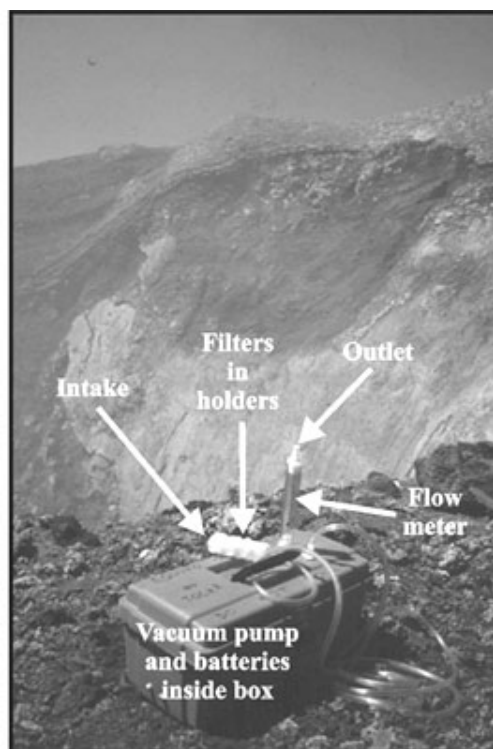
FIG. 1. 'Filter pack' instrument situated on the edge of the summit crater of Villarrica volcano.
