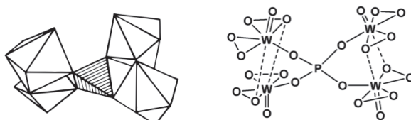
Figure I-4 – The structure of the Ishii-Venturello anion [\text{PO}_4\{\text{W}(\text{O})(\text{O}_2)_2\}_4]^{3-} [30b, 46]
