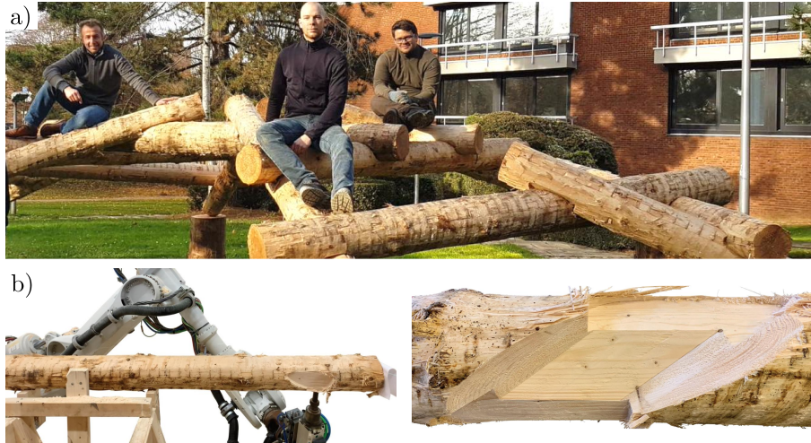
Figure 1.3: a) Log reciprocal structure constructed at UCLouvain (Belgium) presented in Geno et al. [26]. b) Final wood-wood connection cut using a robotic arm.
