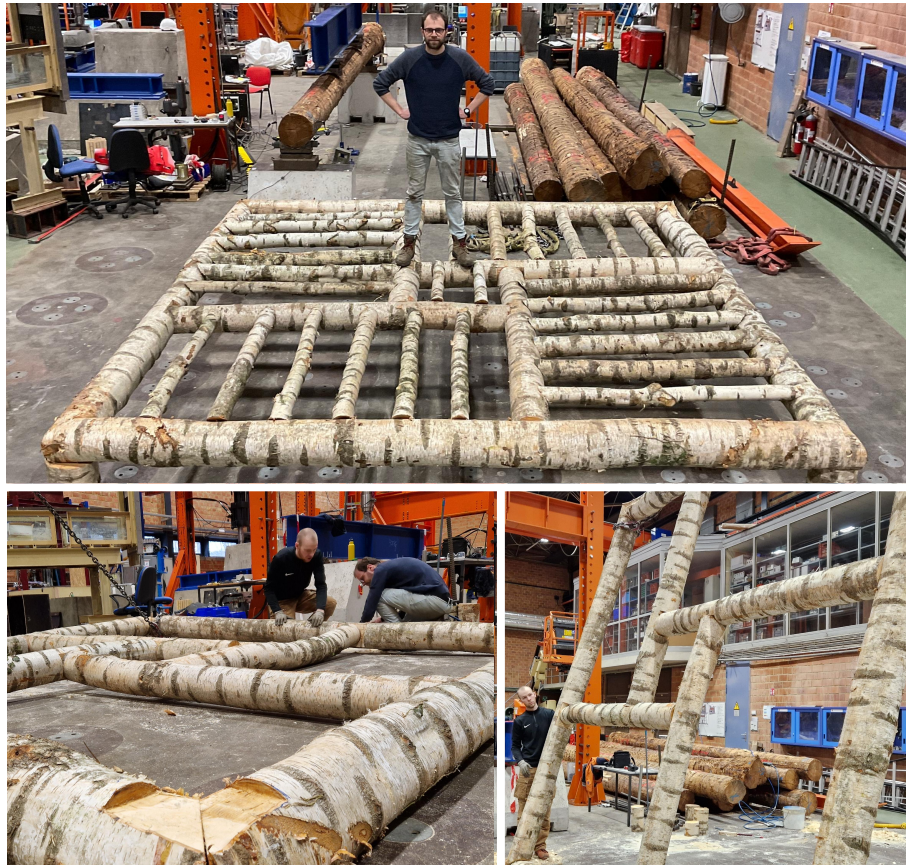
Figure 2.2: Mock-up of a reciprocal log floor 4 m × 4 m (birch wood).
