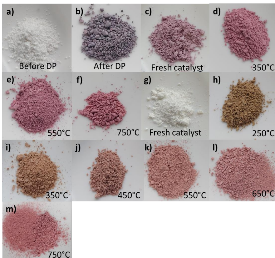
Figure 2.1. Photographs of the different powders synthesized in this work. a) \text{SiO}_2 support used for the deposition – precipitation of gold; b) \text{Au/SiO}_2 DP; c-f) \text{AuSiO}_2\text{-x} ; g-m) \text{AuSiO}_2\text{-MPTMS-x} . The calcination temperature of each sample is mentioned in each image.
