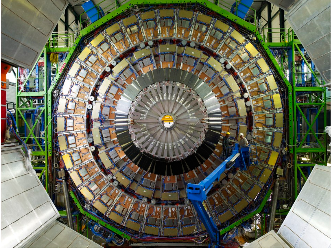
Figure 3. Photograph of the ME1 muon station of the “plus” ( z > 0 ) endcap during the construction of CMS. Visible in concentric rings are the CSC types ME1/2 and ME1/3. The ME1/1 chambers are hidden behind the endcap calorimeters closest to the center. The endcap RPCs are in the layer behind the CSCs.
