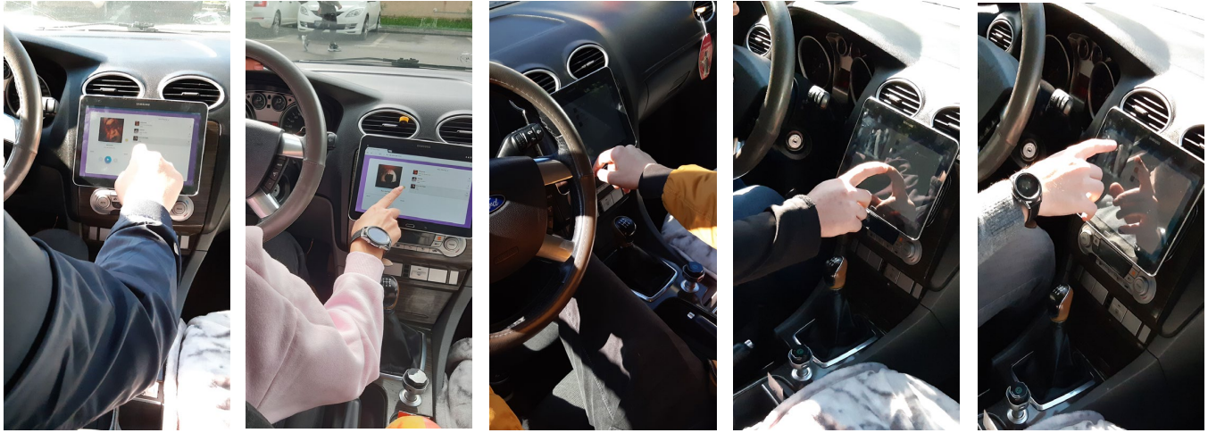
Figure 2: Photographs captured during the usability study of the V2DUI, showing participants using touch input to control a music player application on the in-vehicle infotainment system with vibrotactile feedback delivered on the smartwatch.
